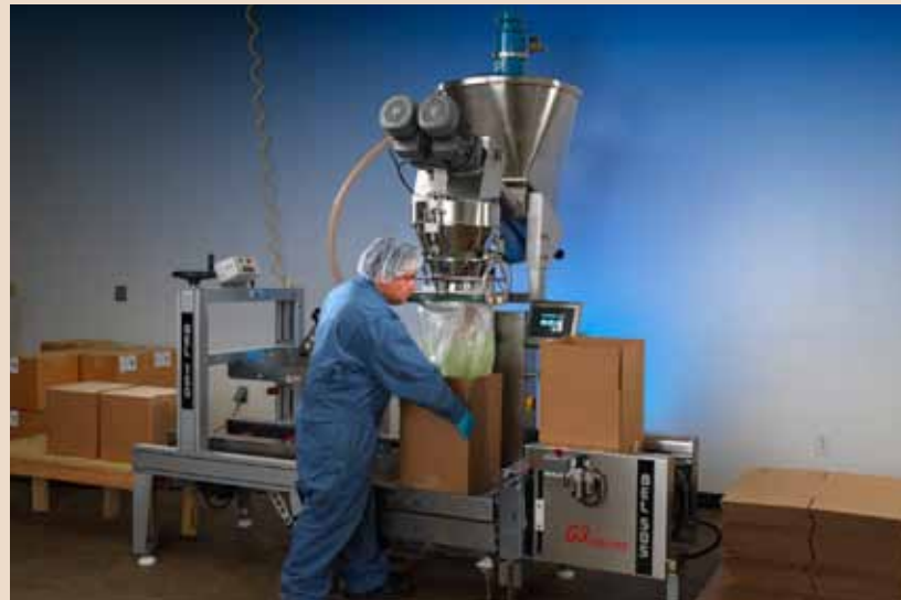
The semi-automated, high-speed weigh packer has the capability to weigh and pack up to 15,000 pounds of product daily.
